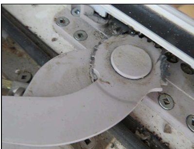
1.7 Item 1(Picture) Stripped gears.
